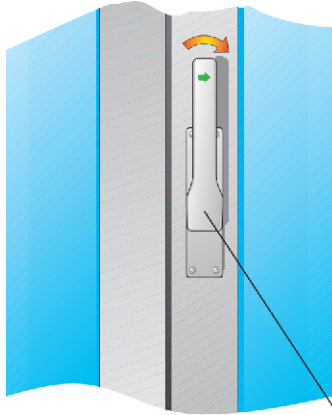
Double-action flush bolt for double-leaf doors. Art. no. 14415 H, 14416 V.
